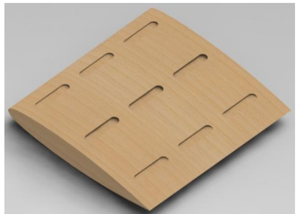
Figure 2.2: Slot type dimple Airfoil
