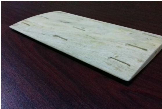
Figure 2.6: Slot type dimple Airfoil
